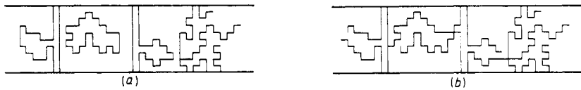
Figure 3. (a) A 40-step padded polygon, a 38-step polygon, a 38-step padded polygon and an unfolded 3-star with 20 steps in each arm. These can be concatenated as in (b), starting with the two 38-step polygons in the middle, to give a brush with v_1 = 3, v_2 = v_3 = 4 .
